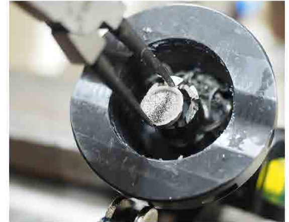
Fig. 9.2 IMPORTANT! REMOVE the slug and swarf with pliers.
