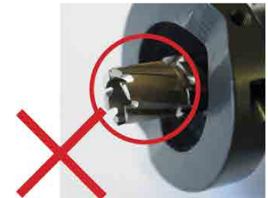
INCORRECT. Installed cutters should NOT remain protruding from the cutter assembly. Ensure that cutters are fully retracted inside the cutter assembly before using the Drill Jig.
