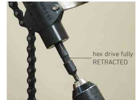
Fig. 8.3 Set drill to reverse and back out the cutters / hex drive until it is fully retracted.
