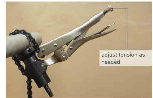
Adjust tension to ensure the clamp body is secure on the rail.
