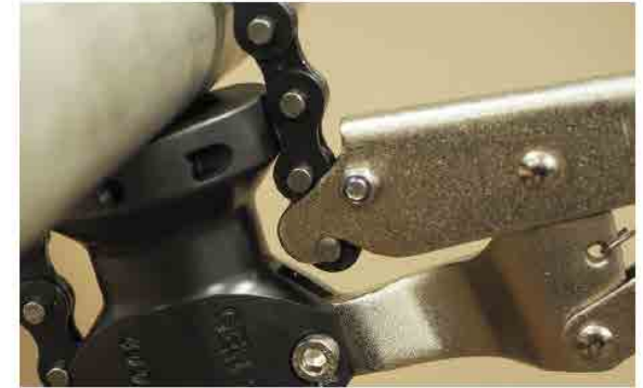
Above: The clamping chain is secure, in a central position, and is not touching the engaged vice grip or the central section of the cutter assembly.
