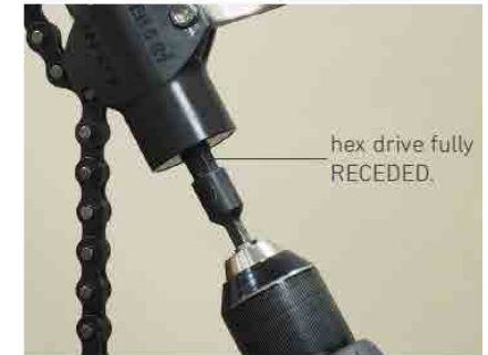
Fig. 8.2 STOP drilling once the hex drive has fully receded inside the Drill Jig.
