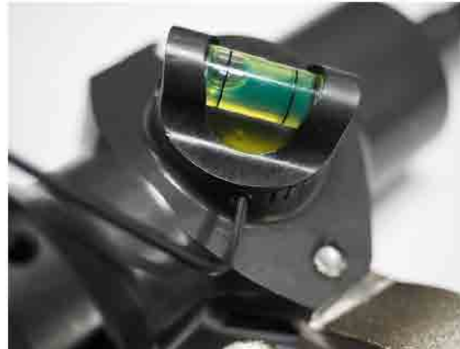
Fig. 4.1 Loosen the two grub screws with the Allen key to adjust the angle setter.
