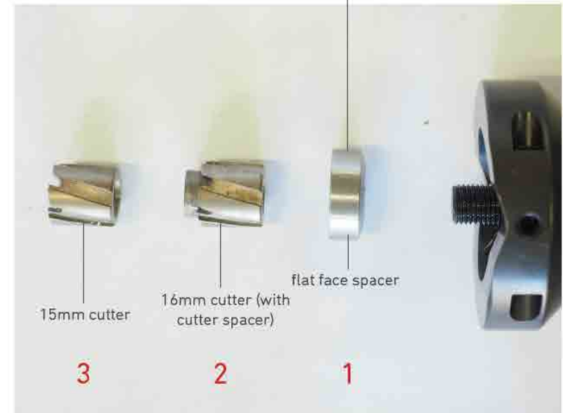
The flat face spacer is installed FIRST, followed by the cutter installation (see step 3). Remember to fully extend the cutter end of the Drill Jig (as shown).
