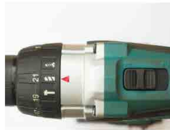
Above: Our example drill is set to: "Drill"; high torque; and LOW speed (1)
