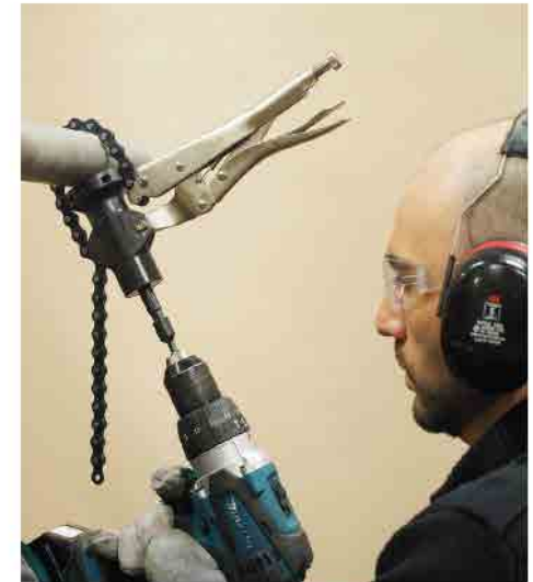
Above: The G5 Drill Jig in use. Proper use of the Drill Jig will result in a significantly faster and more professional finish.
