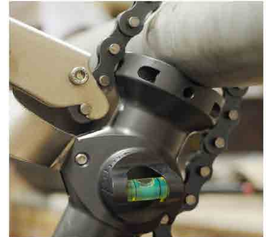
Above: The drill Jig's spirit level bubble should be centred before drilling to enable consistent angle drilling at your set angle.
