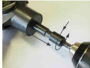
Fig. 2.1 If cutters are pre-installed, use your drill to ensure that both the hex drive and cutter end of the cutter assembly are fully retracted.
