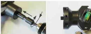
Fig. 3.1 Use your drill to fully extend the cutter end (above right) BEFORE cutter installation.
